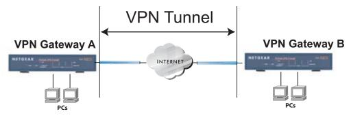
Figure C-5: VPN tunnel Security Associaton (SA)
